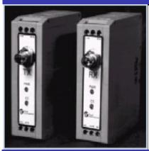
The FOR-CC Contact Closure Output Module provides Form-C relay output connections that change state (open/closed) based on the state of the input contacts supplied to the partnered FOT-CC Contact Closure Input Module. The input information is transferred to the FOR-CC over a single fiber. LED Indicators on the FOR-CC provide visible monitoring of the operating power and the state of the output contacts.
